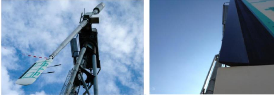
Figure 2-1: Test rig at DTU test field with blade section 2.2m spanwise length and 1m chord
